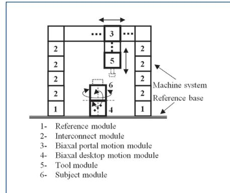
Figure 4. Reference assembly machine system
