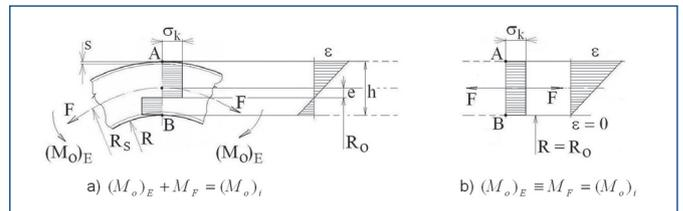
Figure 12. Distribution of stresses and engineering strains
