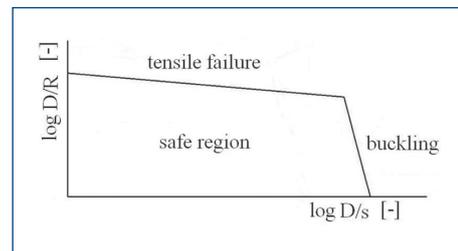
Figure 4. Technological forming limit diagram (TFLD)
