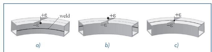
Figure 5. Correlation between the strain distribution and weld position
