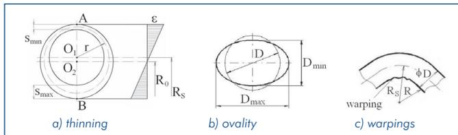
Figure 3. Failures of round tubes after bending
