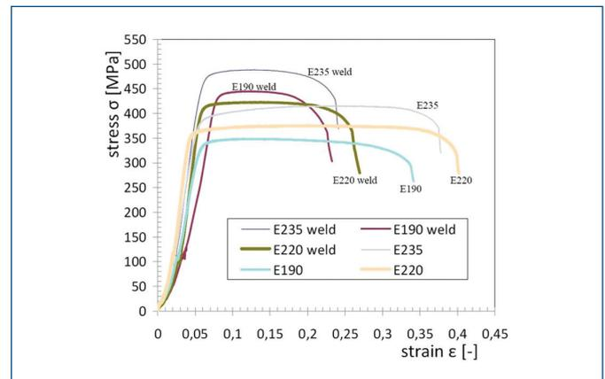
Figure 2. Results of tensile test
