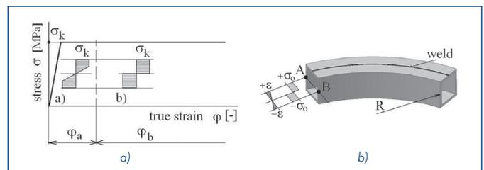
Figure 8. Linear approximation of the flow stress
