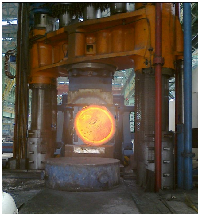
Figure 1. View inside working space of hydraulic press with two columns
