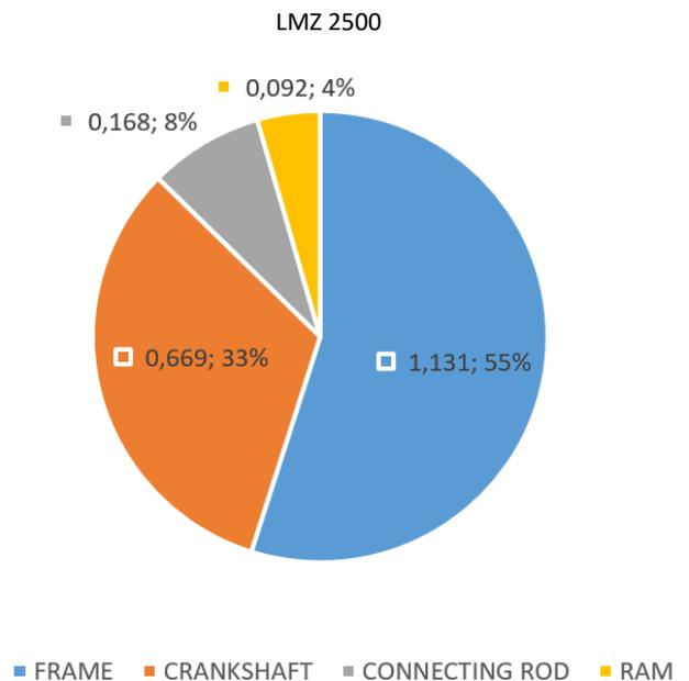
Figure 10. Representation of displacement in existing design of forging press
