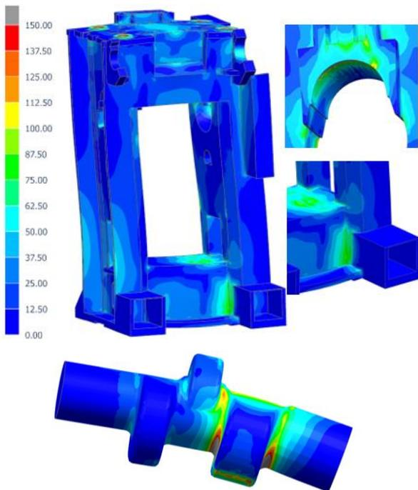
Figure 8. Stress distribution in parts of forging press
