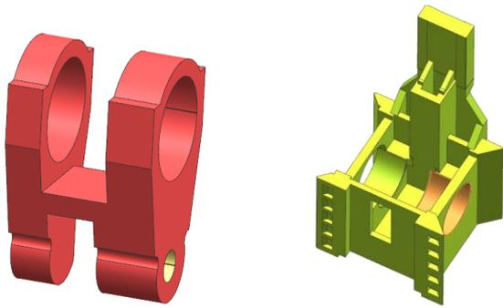
Figure 7. Reinforcement of ram and connecting rod
