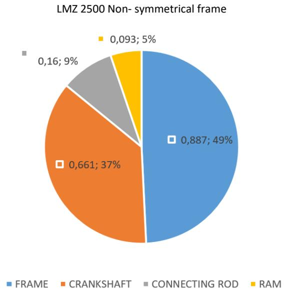
Figure 9. Representation of displacement in new design of forging press
