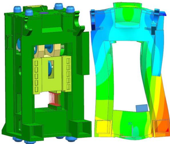
Figure 4. Tilting of tool (die) during eccentric loading (magnified deformation)
