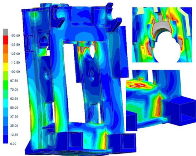
Figure 3. Extremely loaded frame during eccentric loading (original solution) (MPa)
