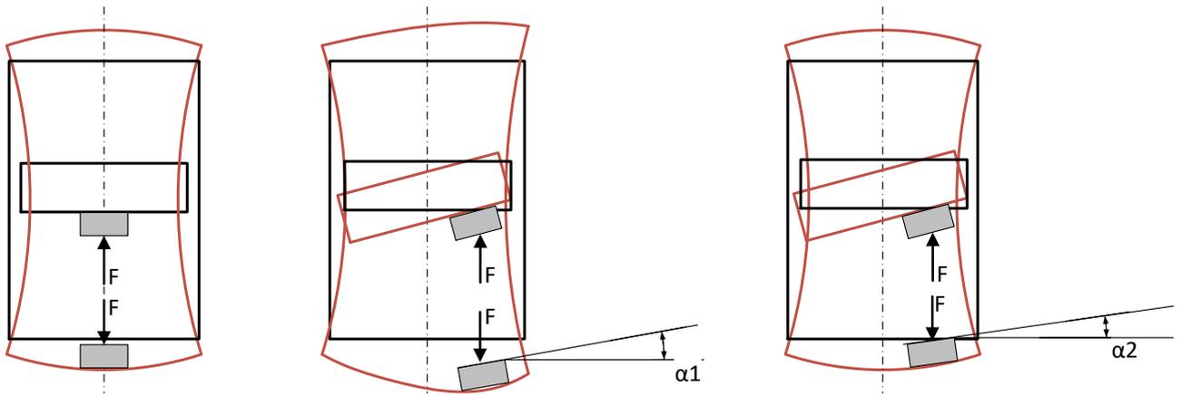
Figure 2. Tilting of tool under various loading- from the left is centric forging, eccentric forging on symmetrical frame and eccentric forging on non-symmetrical frame
