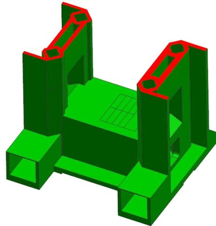
Figure 5. Reinforcement of frame on side of forging force
