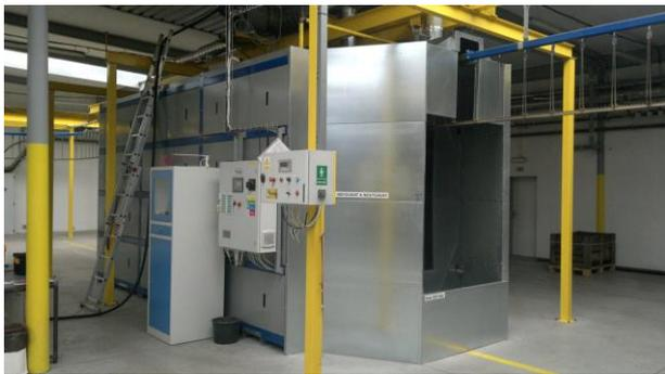
Figure 2: Catalytic infrared kiln
