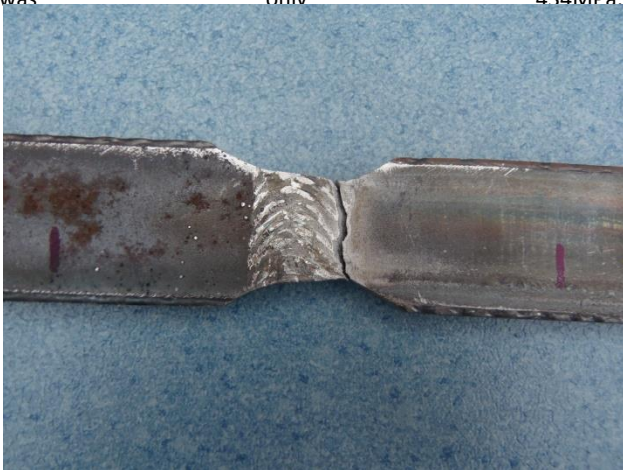
Figure 4. Specimen failure – fracture in the HAZ on S355
