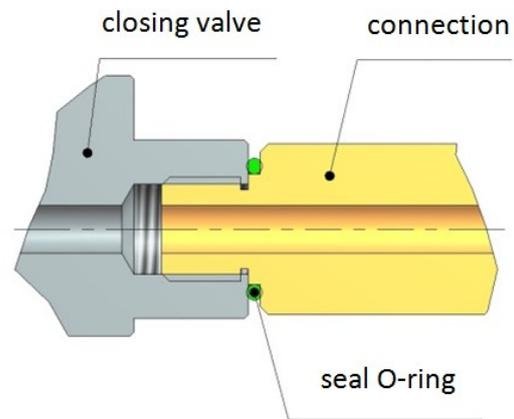
Figure 4. Seal between the connection and closing valve – cross section
