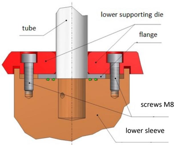
Figure 2. Fixing of tube ends – cross section
