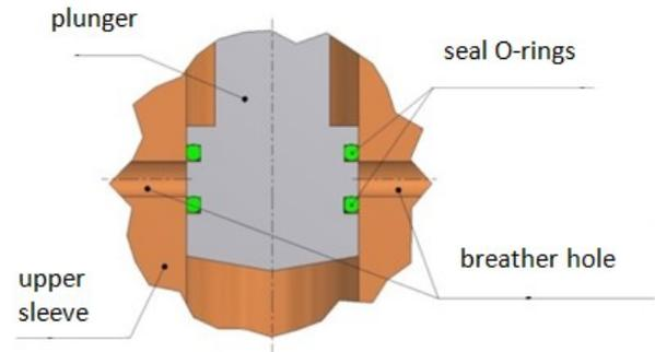
Figure 3. Plunger seal – cross section
