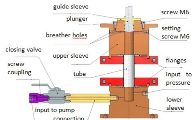
Figure 5. Filling and venting system
