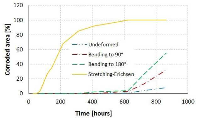
Figure 10. Corroded surface-Time dependence for GA1 samples with Zn-Al-Mg coating
