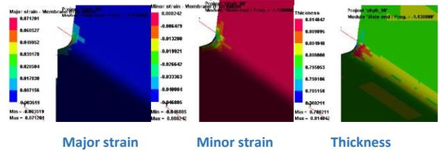
**Figure 6.** Strains calculated by numerical simulation when bending to 90° – critical major/minor strains [0.07; 0.0002]
