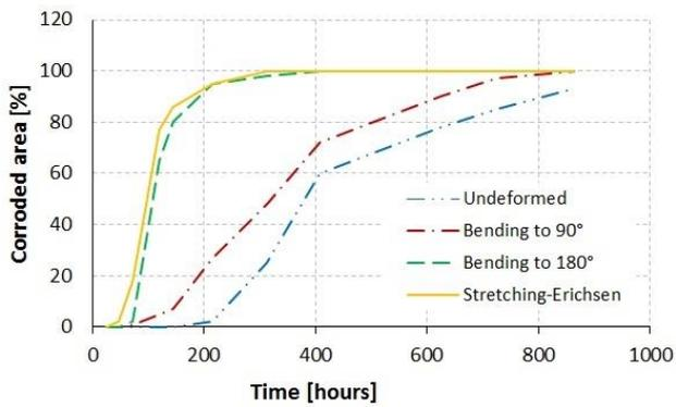
Figure 8. Corroded surface-Time dependence for GI samples with Zn coating
