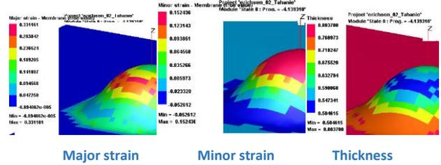
**Figure 5:** Strains calculated by numerical simulation when stretching by Erichsen test – critical major/minor strains [0.33; 0.15]
