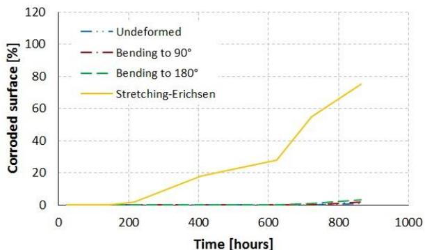
Figure 12. Corroded surface-Time dependence for GA2 samples with Zn-Al-Mg coating
