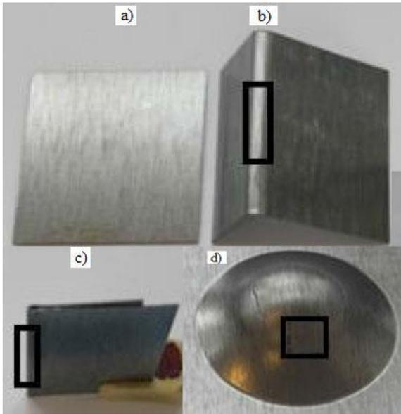
**Figure 3.** The specimens shape after plastic deformation a) no deformation, b) bending 90°, c) bending 180°, d) stretching by Erichsen test
