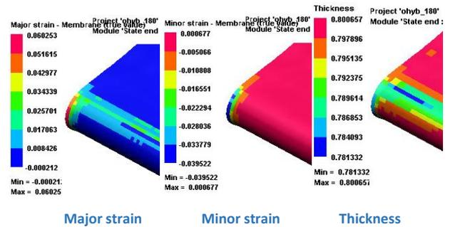
**Figure 7.** Strains calculated by numerical simulation when bending to 180° – critical major/minor strains [0.07; 0.0007]
