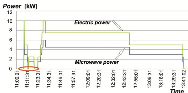
Figure 8. Power demand profile of the HR-Lab
