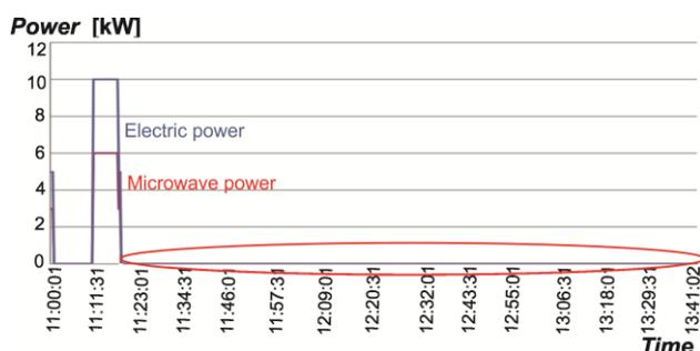
Figure 9. Power demand profile of the microwave reactor MOS
