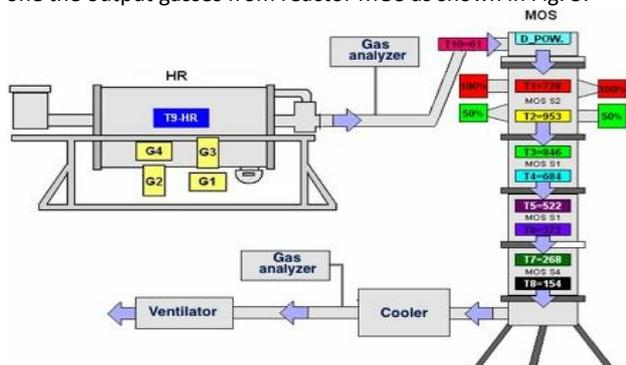
Figure 3. Setup for tires gasification experiment
