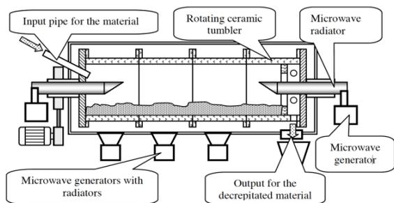
Figure 1. Scheme of microwave reactor Aton HR
