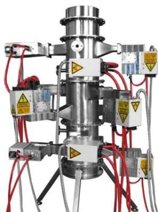
Figure 2. MW reactor MOS with 3 sections
