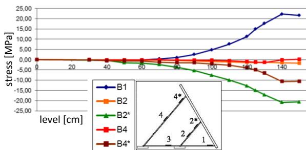
Figure 8. Illustration of the results of the tensometric measurement of stress, in dependence on the water level [Soos 2014a]
