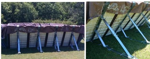
Figure. 10 Modular flood barrier structure – test basin at TOP 2016
