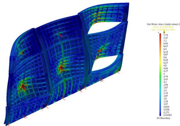
Figure 4. Finite element method FEM analysis of the arrangement of plastic block loading [MPa]
