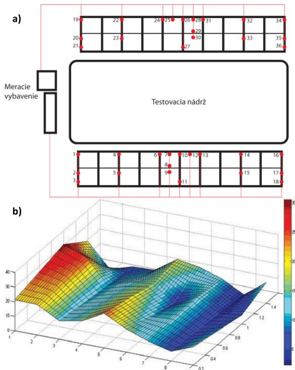
Figure 9 a) Measurement scheme. b) Experiment of the failure one steel support part - demonstration of the measurement results of collapsing wall deformation measuring [cm] [Kopunec 2015].
