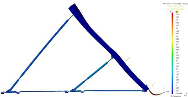
Figure 5. Finite element method FEM analysis of back construction loading [MPa] (def. M 20:1)
