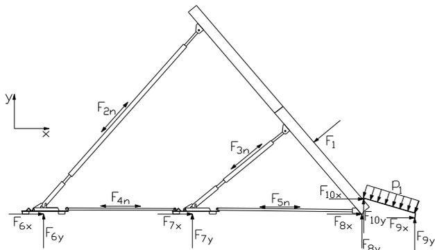
Figure 6. Graphic interpretation of the complex FEA simulation reaction of our solution design.
