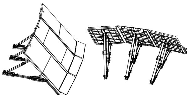
Figure 1. Modular flood barrier structure
