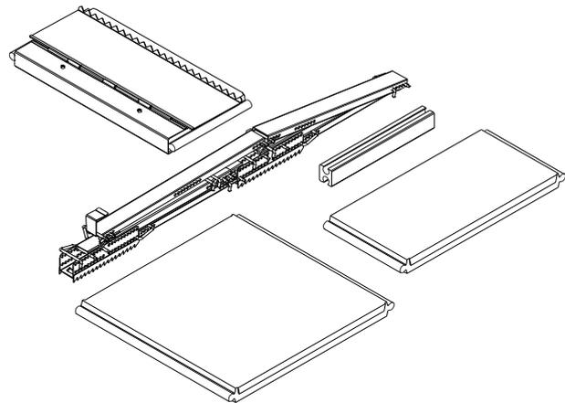
Figure 11. Basic parts of the modular structure of walls in disassembled state before assembly
