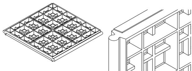
Figure 12. Newest shape of the monolith blocks with vertical and horizontal locks.
