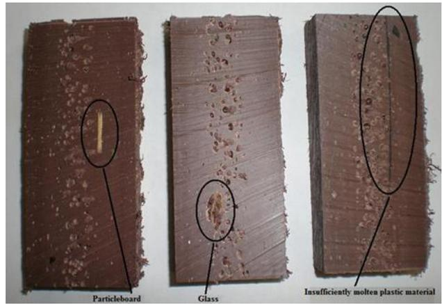
Figure 11. Impurities in plastic boards from recycled plastic
