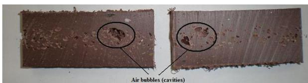
Figure 10. Bubbles in a plastic plate
