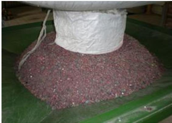
Figure 8. Crushed and sieved plastic waste
