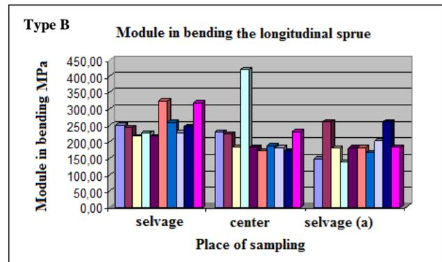
Figure 18. Modulus in flexural test specimen, type A and type B
