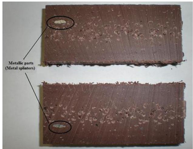
Figure 12. Metal chips in the plastic plate from recycled plastic
