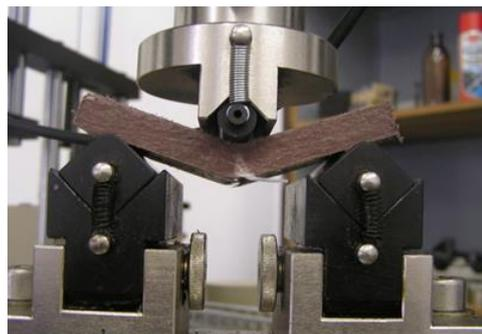
Figure 13. Damage of the test specimen during the bending test, test I
