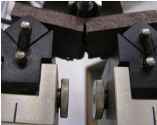
Figure 15. Damage of the test specimen at bending, test III
