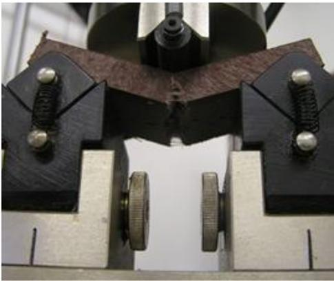
Figure 14. Damage of the test specimen at bending, test II
