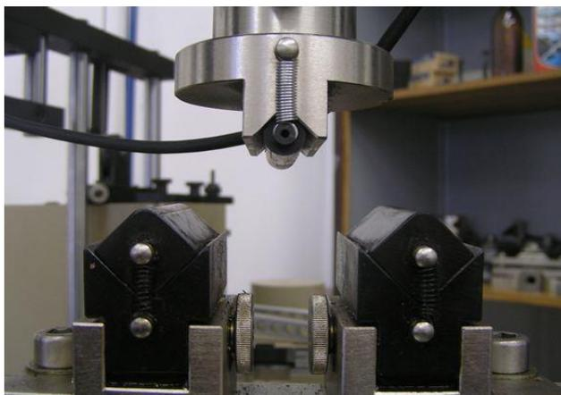
Figure 3. The bending tool in the a basic position
