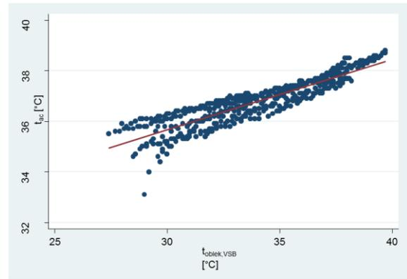
Figure 7. The relationship between the body temperature  $t_{ac}$  (measured in the ear canal) and the under suit temperature measured by the SAM device
