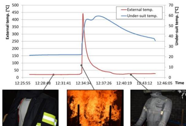
Figure 9. Test result at firefighter's suit mannequin test (Spain)
