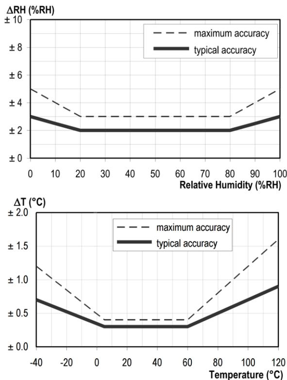
Figure 13. Accuracy of the internal sensor (SHT21)
