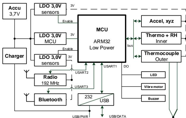
Figure 2. Functional diagram of measurement device
