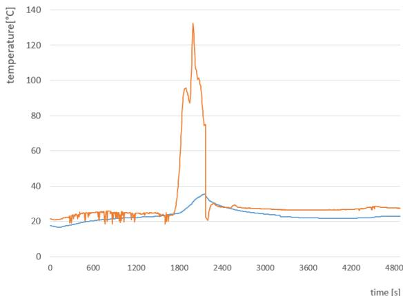
Figure 12. Flashover test result – external and internal temperatures
