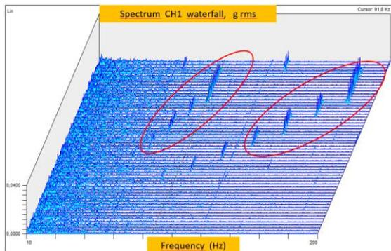
Figure 7. Frequency spectrum of machine №.2 [Team 2016]
