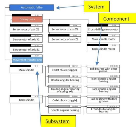
Figure 4. Example of machine breakdown [Team 2016]
