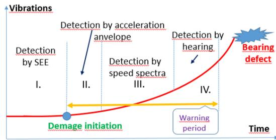
Figure 8. Progress of bearing defects
