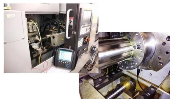
Figure 5. Lathe examined in preparation for diagnostics (top photo) and mounting of sensors (bottom photo) [Team 2016]
