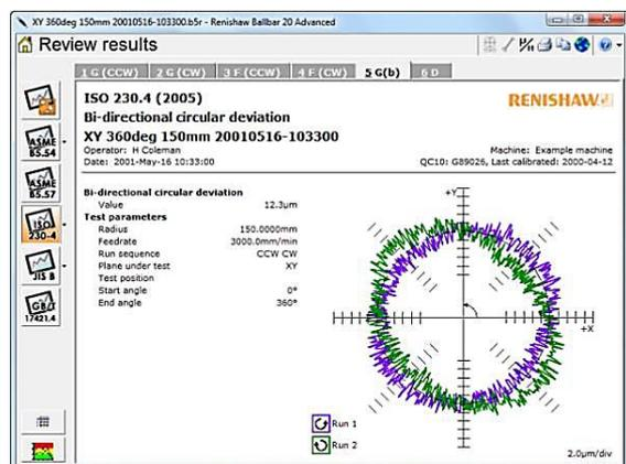
Figure 3. Example of measurements of bi-directional circular deviation by the program Renishaw 30 [Team 2016]
