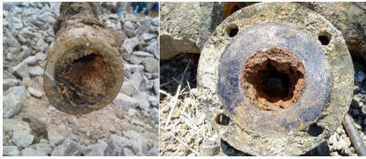
**Figure 5** Repairing of pipelines' failure - cast iron pipe DN100 from 1965, encrustations of the internal surfaces
