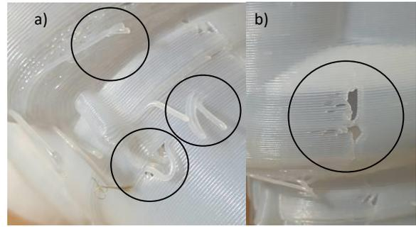
**Figure 9.** Defects of final 3D printed polystyrene pattern, a) various shape errors due to incorrect thread join, b) broken contour resulting in a vertical crevice
