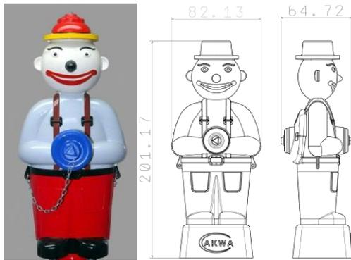
Figure 1. The test product made in the studies and its main dimensions
