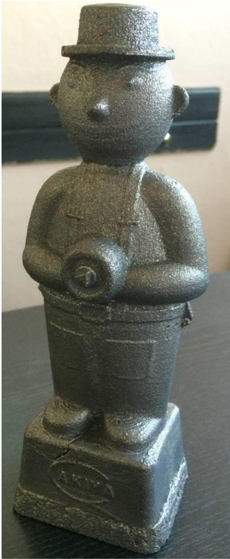
**Figure 8.** Obtained cast iron casting, with visible defects (fracture at the base)
