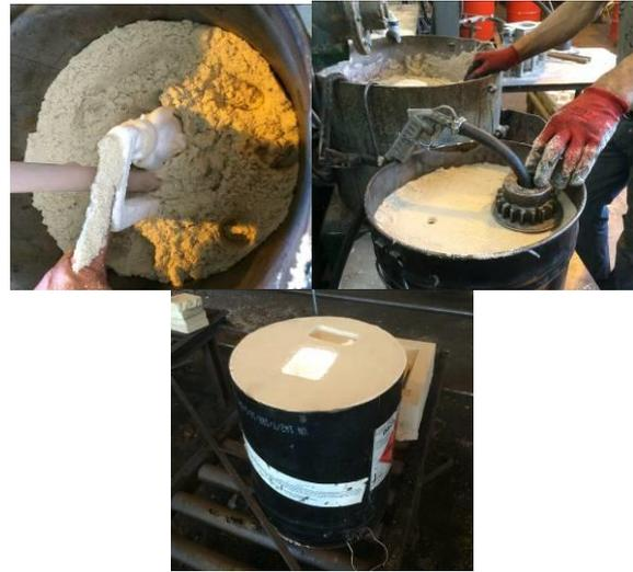
**Figure 6.** Making the quartz sand mold
