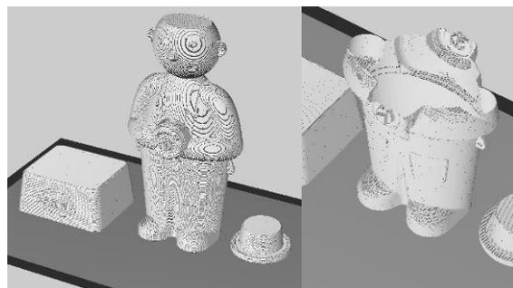
Figure 3. Visualization of the 3D printing program no. 2 – visible machine path and empty infill
