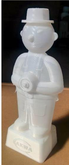
**Figure 4.** Final lightweight polystyrene pattern manufactured using the FDM technology
