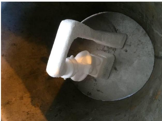
**Figure 5.** The polysterene pattern with the gating system, placed in the molding box
