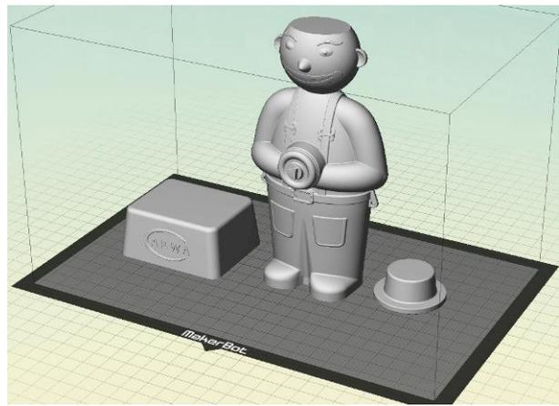
Figure 2. Divided mesh of the product prepared for 3D printing program generation
