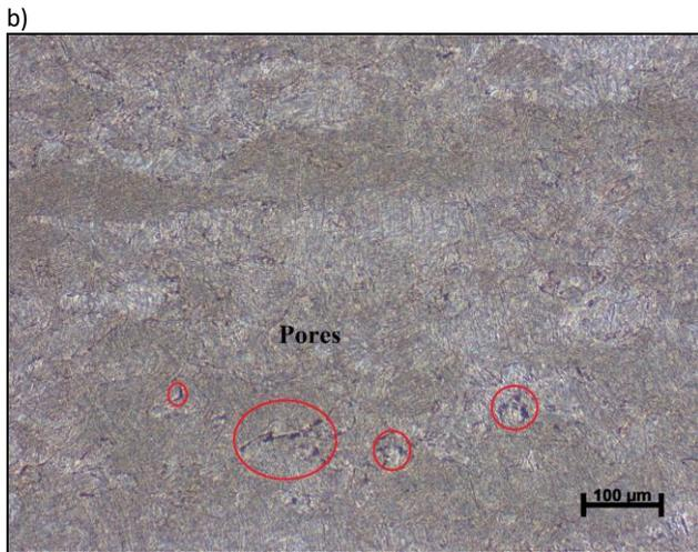
Figure 5 a) Microstructure of Ti6Al4V from OM b) Microstructure of Ti6Al4V from OM with DIC filter outlining the pores
