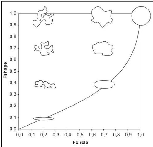
Figure 2. The pores shapes in depending on  $f_{shape}$  and  $f_{circle}$ .
