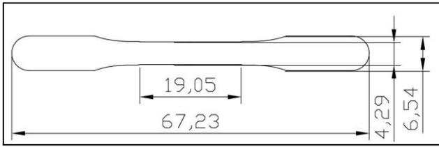
Figure 1. Dimension of sample for static tensile test prepared by LS technology
