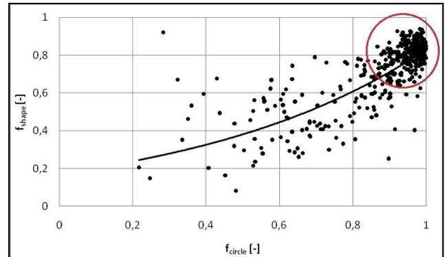
Figure 7. Dependence  $f_{circle}$  vs.  $f_{shape}$ . In red circle are ideal shape pores
