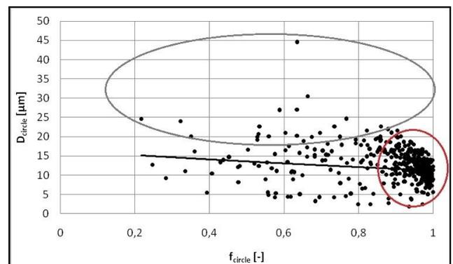
Figure 8. Dependence  $f_{circle}$  vs.  $D_{circle}$ . In red circle is the average pore size. In gray circle are pores with a higher diameter
