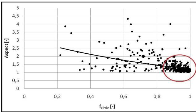
Figure 9. Dependence  $f_{circle}$  vs. Aspect. In red circle are pores that are close to the ratio of 1
