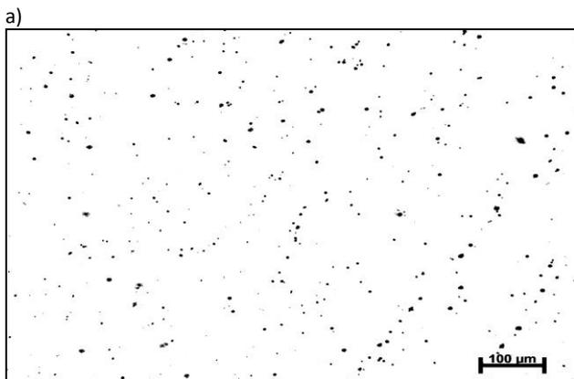
Figure 6 a) Microstructure of Ti6Al4V from OM, not etched b) Microstructure of Ti6Al4V from OM with grid in ImageJ  $\langle x, y \rangle$
