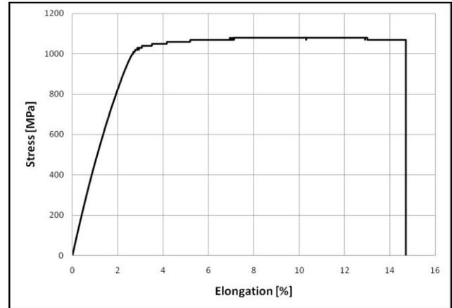
Figure 4. Diagram from the static tensile test
