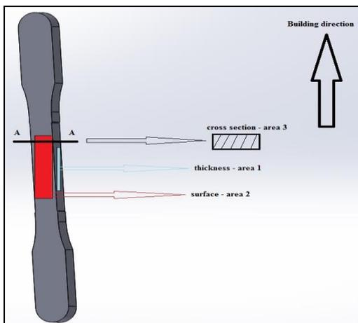
Figure 3. The schematically divided sample into three areas.
