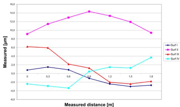
Figure 7. Measured precision values of the guideways on the column [Ucen 2014]
