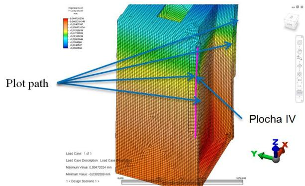
Figure 11. Plot path edges [TOSHULIN 2014]
