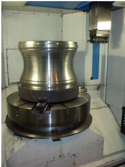
Figure 3. Vertical turning machining centre [TOSHULIN 2014]
