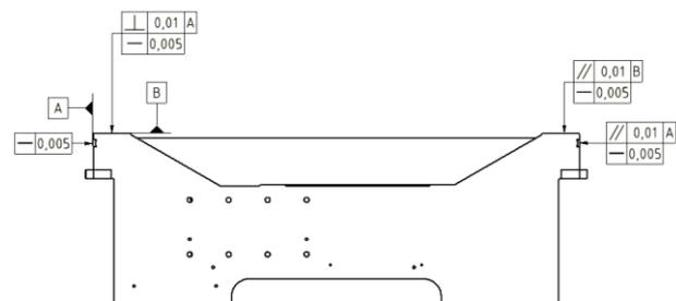
Figure 6. Examples of precision of ground faces [Ucen 2014]
