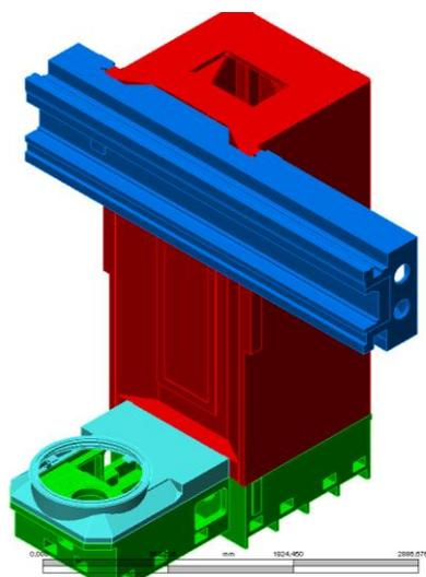
Figure 4. CAD model of the machine-tool frame [Ucen 2014]
