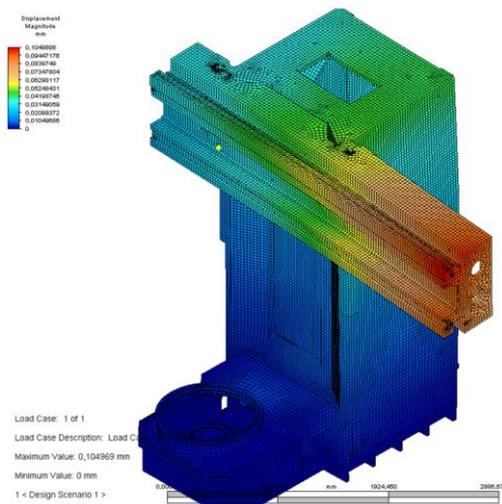
Figure 10. Deformation of the frame (Var. No. 2) [TOSHULIN 2014]
