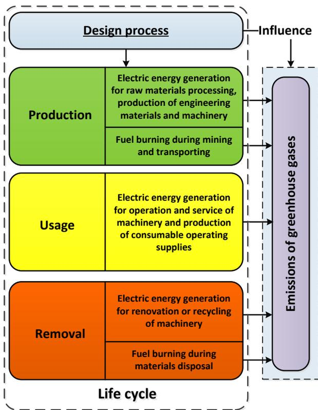
Figure 1. Lifecycle of the machinery and its impact on the environment
