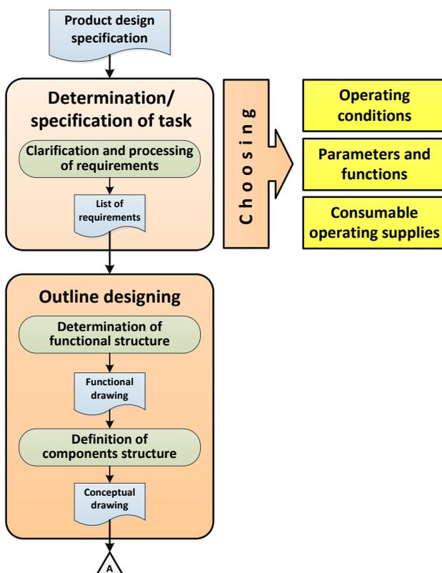
Figure 2. Design process of machinery [Blecha 1999]
