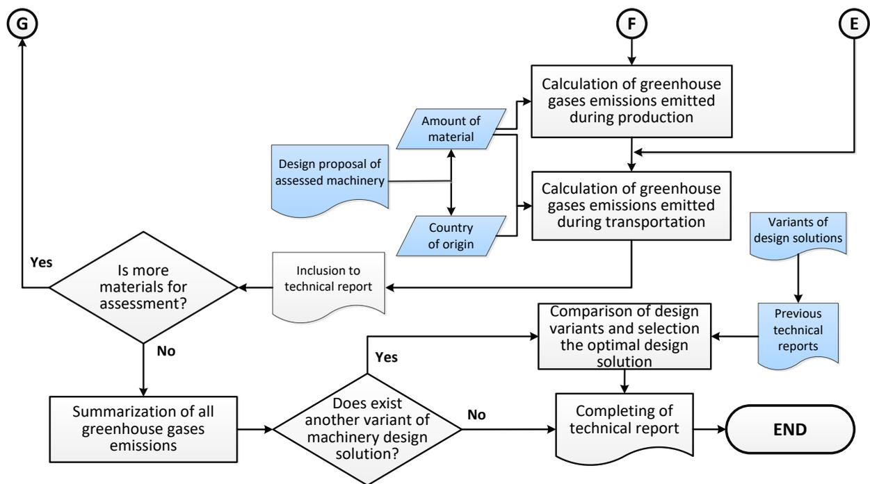
Figure 4. Methodology for assessment of GHG emissions released throughout production of engineering materials (to be continued)
