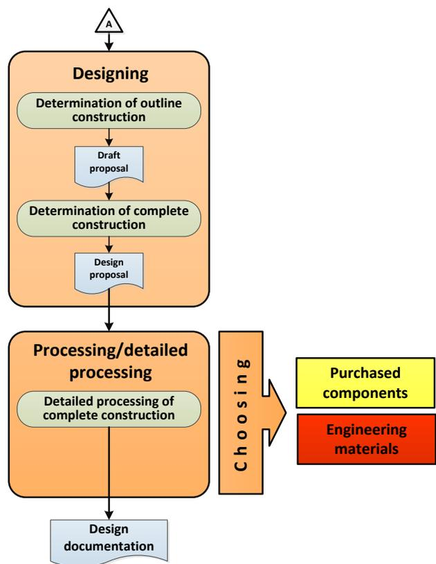
Figure 2. Design process of machinery [Blecha 1999] (to be continued)
