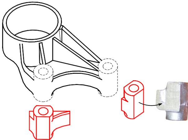
Figure 1. Sampling points of the castings for hardness research
