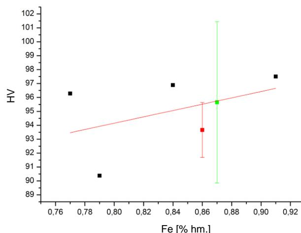
Figure 5. Hardness of the sample B with the respect to the Fe content
