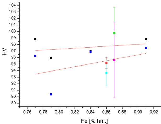
**Figure 7.** Hardness of the sample B(B720) with the respect to the Fe content
