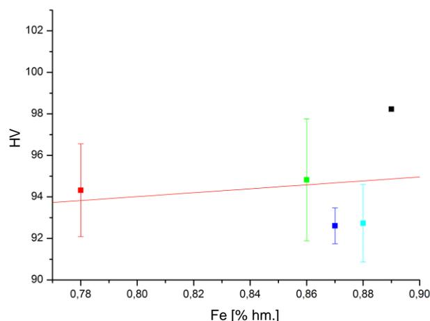
Figure 6. Hardness of the sample D with the respect to the Fe content
