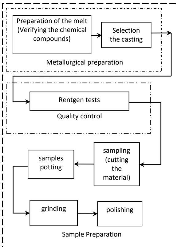
Figure 2. Scheme of samples preparing for the micro hardness measurement
