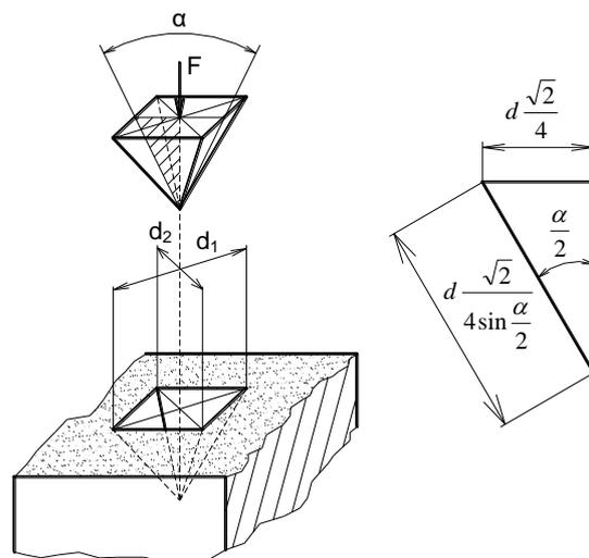
Figure 3. Scheme of Vickers hardness measurement
