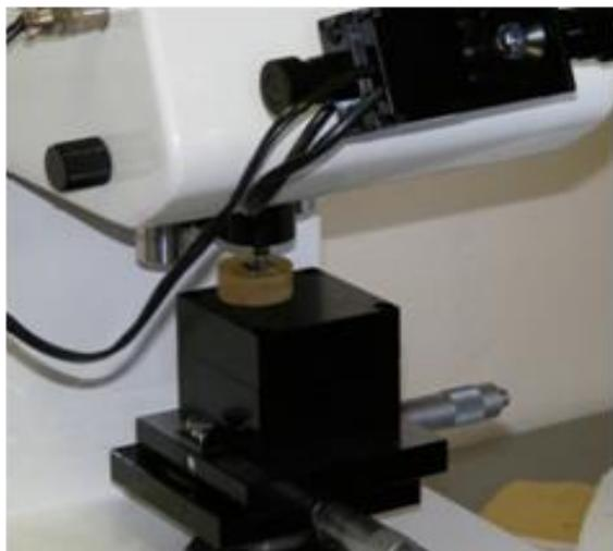
Figure 4. Digital microhardness tester CV - 400D
