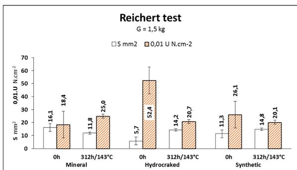
**Figure 2.** Influence of temperature stress on lubricity and load-carrying capacity of engine oil film
