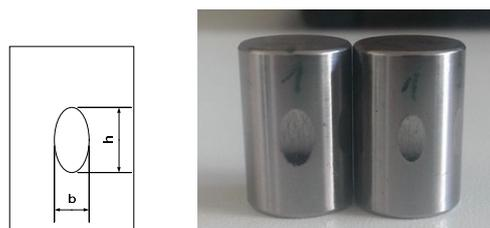
Figure 1. Reichert test – schematic for wear area calculation and view of cylinder rolls exposed to test
