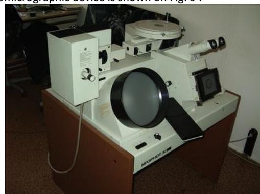
Figure 9. Optical microscope NEOPHOT 32
