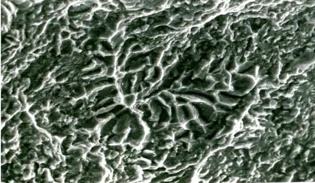
Figure 3. Mechanism of  $\alpha$  - phase dendrites and eutectic disturbance/250x/
