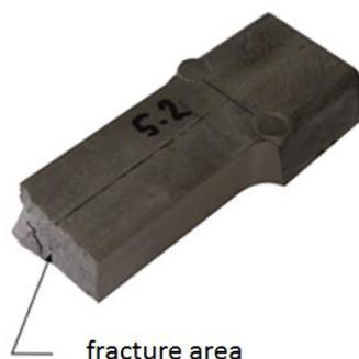
Figure 1. Test rod with the fracture area
