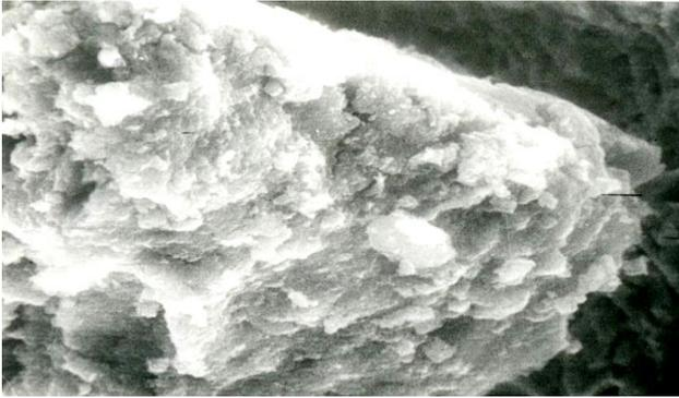
Figure 7. Cluster of Al<sub>2</sub>O<sub>3</sub> particles
