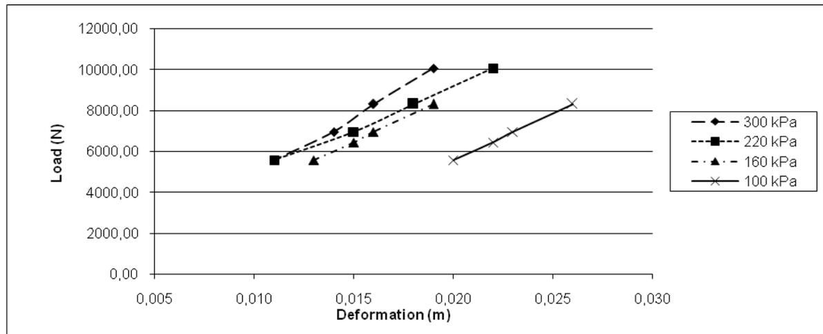
Figure 2. Radial deformation characteristic of the Mitas TS05 10.0/75-15.3 PR10 tire
