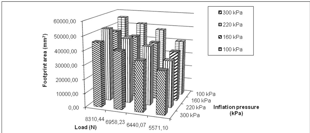
Figure 3. Dependence of the tire print area on the vertical load and inflation pressure
