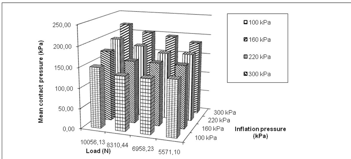
Figure 4. Dependence of the mean tire contact pressure on the load and inflation pressure
