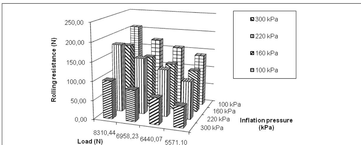
Figure 5. Dependence of tire rolling resistance on the load and inflation pressure
