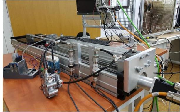
Figure 4. Device for testing of the ball screw drive
