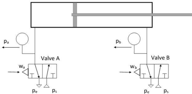
Figure 2. Pneumatic scheme of the load system
