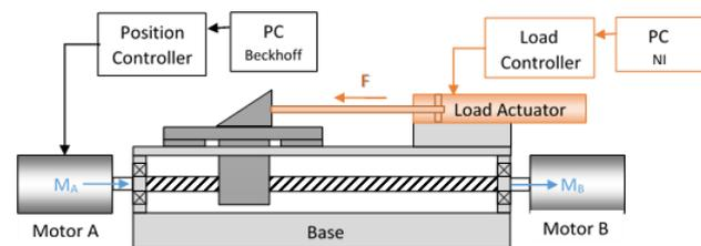
Figure 1. Scheme of the experimental equipment for testing of the linear drive with ball screw
