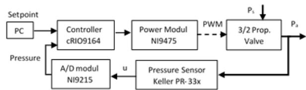
Figure 3. Proportional valve control system scheme
