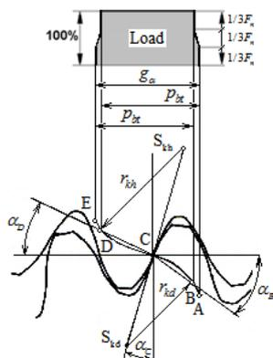
Figure 4. Allocation  $F_n$  along mesh in C-C gearing
