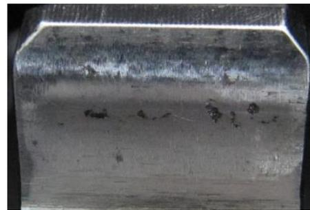
Figure 6. Pitting in the standard involute gearing
