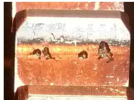
Figure 7. Pitting in the C-C gearing
