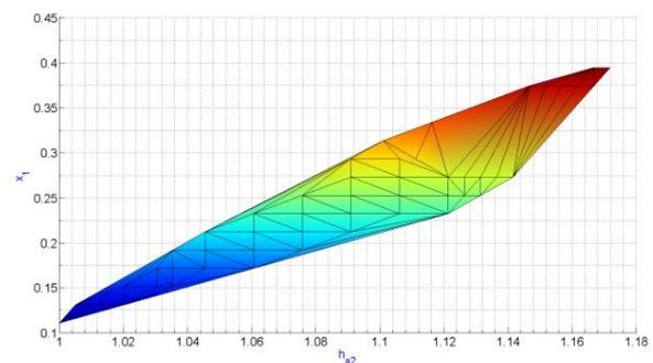
Figure 13. Optimal values  $h_{a2}$ ,  $x_1$  for maximum contact load capacity depending on  $\varepsilon_\alpha$
