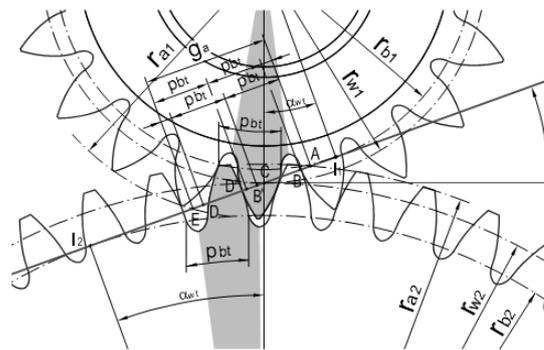
Figure 1. Geometry of involute HCR gearing
