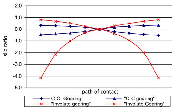
Figure 3. Slip ratio of involute HCR and non-involute C-C gearing along the contact path
