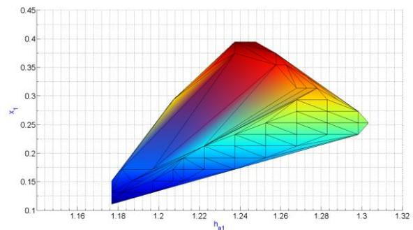
Figure 12. Optimal values  $h_{a1}$ ,  $x_1$  for maximum contact load capacity depending on  $\varepsilon_\alpha$
