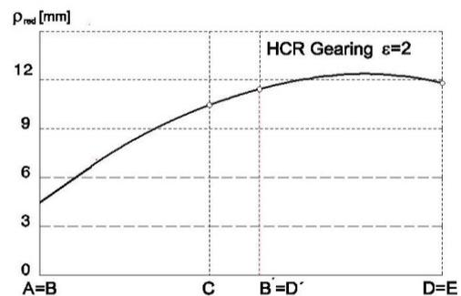
Figure 9. Mean contact radius of curvature along the contact path of HCR gearing
