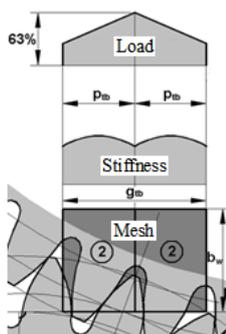
Figure 5. Allocation  $F_n$  along mesh in HCR gearing
