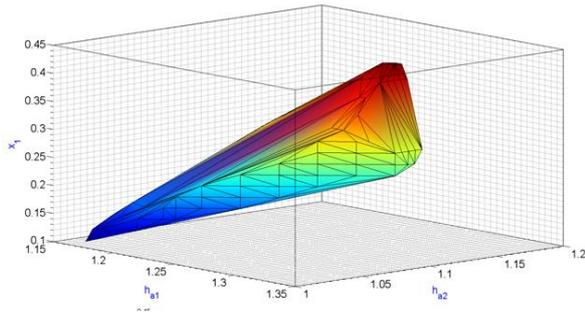
Figure 14. Optimal values  $h_{a1}$ ,  $h_{a2}$ ,  $x_f$  for maximum contact load capacity depending on  $\epsilon_\alpha$
