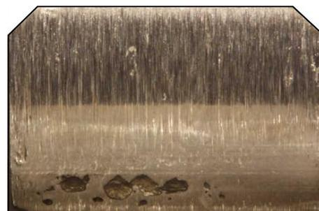
Figure 8. Pitting in the nonstandard involute gearing (HCR)
