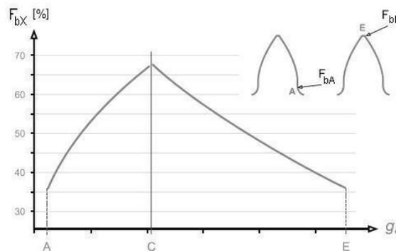
Figure 2. Shape of the curves representing the load along the path of contact in one pair of HCR gearing teeth
