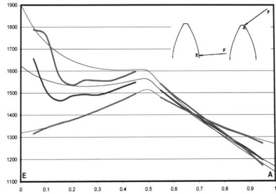
Figure 11. Contact stress of HCR gears along the contact path for various geometry characteristics of gearing
