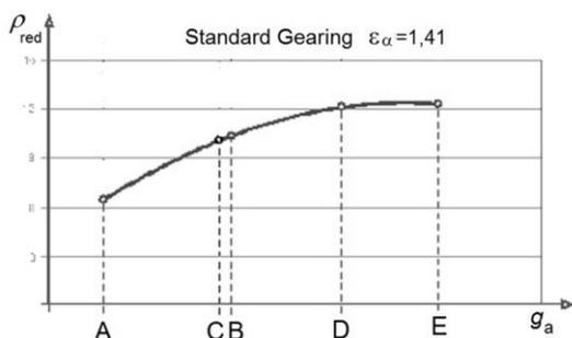
Figure 10. Mean contact radius of curvature along the contact path of standard involute gearing
