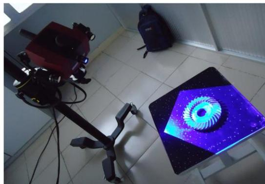
Figure 6. Scanning the machined gear.
