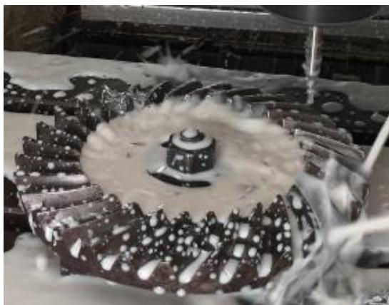
Figure 5. Cutting the designed gear on a 3-axis machining center.
