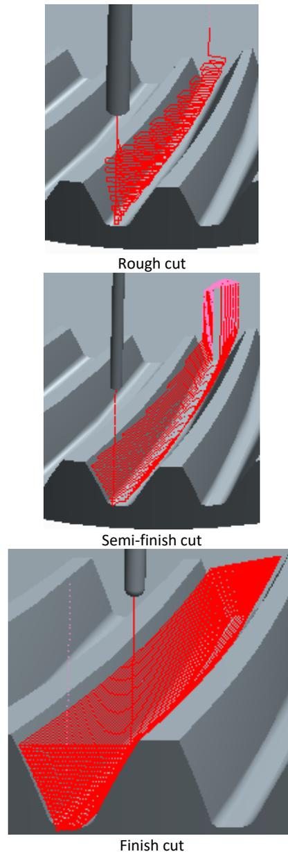
Figure 3. Tool paths for gear cutting.
