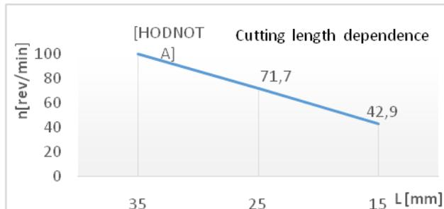
Figure 7. Dependence of the cutting substance length on revolutions of the feeding roller
