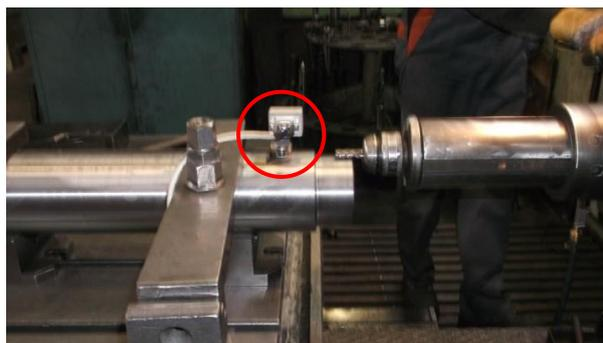
Figure 2. Measurement of vibration at the work-piece
