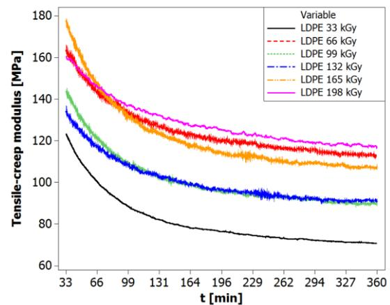
Figure 7. Tensile-creep modulus of irradiated LDPE
