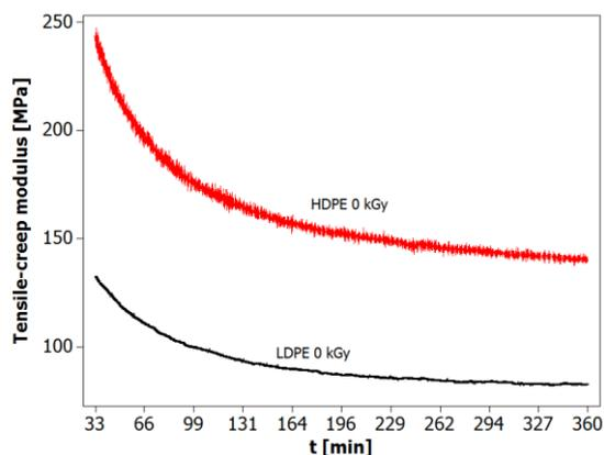
Figure 6. Tensile-creep modulus of HDPE and LDPE
