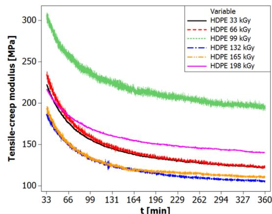
Figure 8. Tensile-creep modulus of irradiated HDPE
