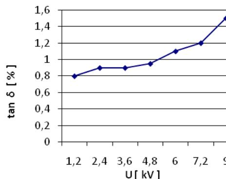
**Figure 4.** Process tan δ loss factor – insulation Calmica 70 0867; t = 1,6 mm
