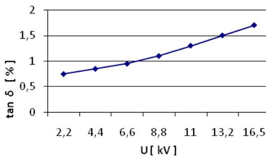
Figure 5. Process tan δ loss factor – insulation Calmica 70 0867; t = 2,3 mm
