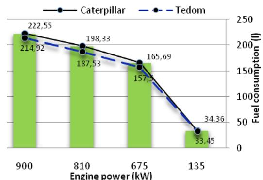
Figure 3. Comparison of fuel consumption in relation to engine power
