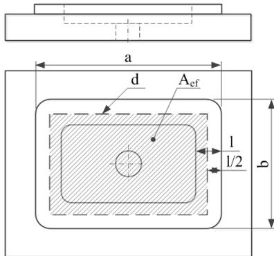
Figure 2. Dimensions of HS pocket [Lazak 2016]
