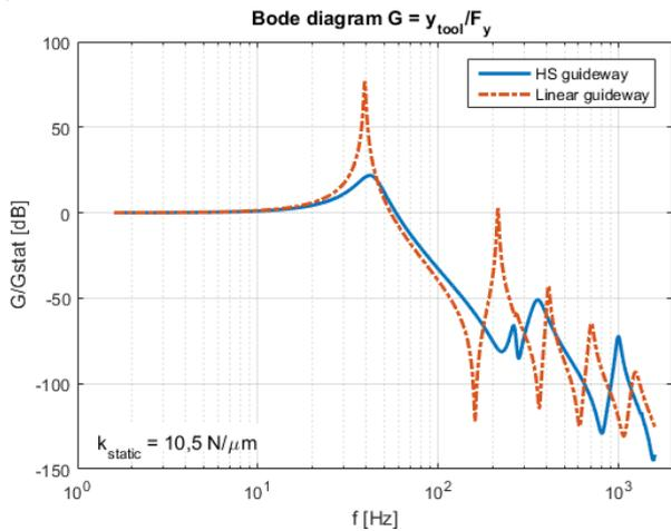
Figure 6. Transfer curve of tool center point deflection with respect to horizontal force
