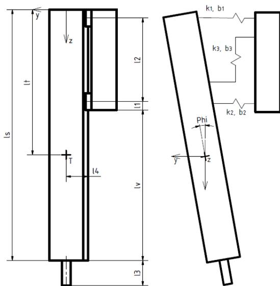
Figure 3. Model of machine tool ram
