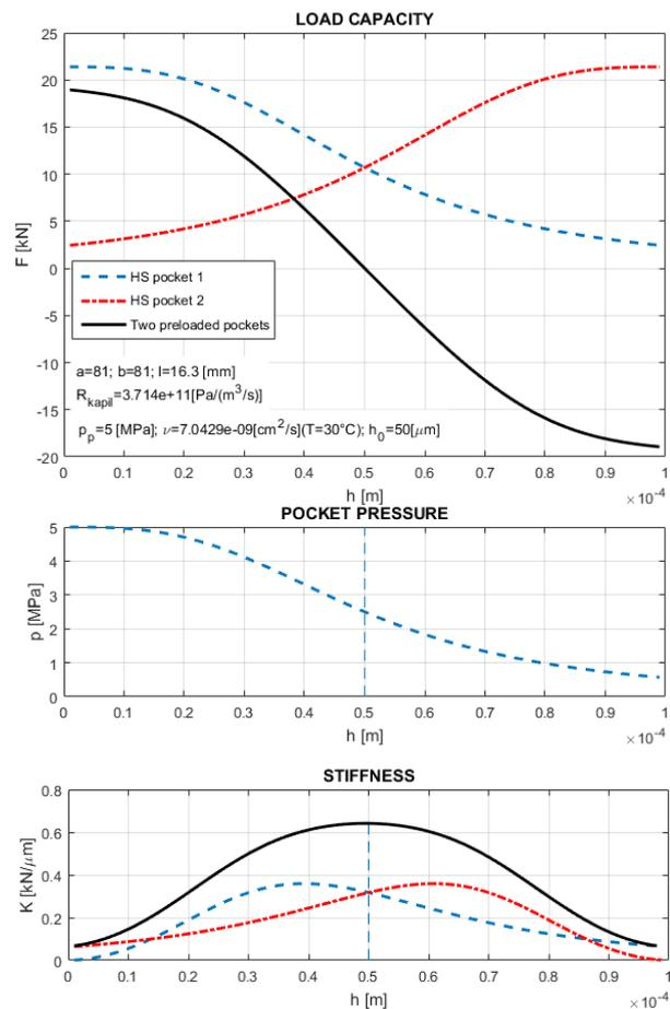
Figure 5. HS pocket parameters
