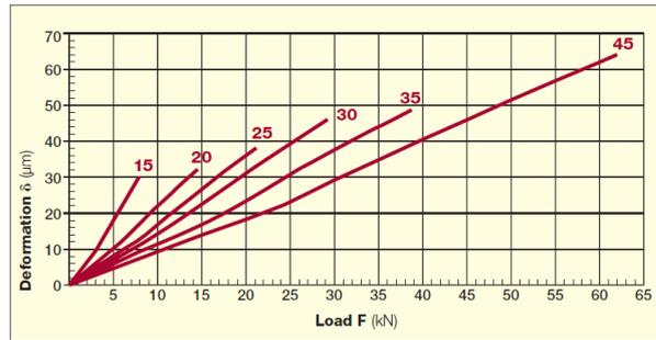
Figure 4. Load-deflection relation of guideway carriage (the red numbers indicate the size of the guideway) [Schneeberger 2017]
