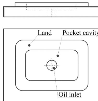
Figure 1. Hydrostatic pocket [Lazak 2016]
