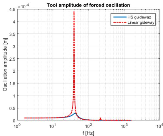
Figure 7. Amplitude of tool center point forced oscillations deflection
