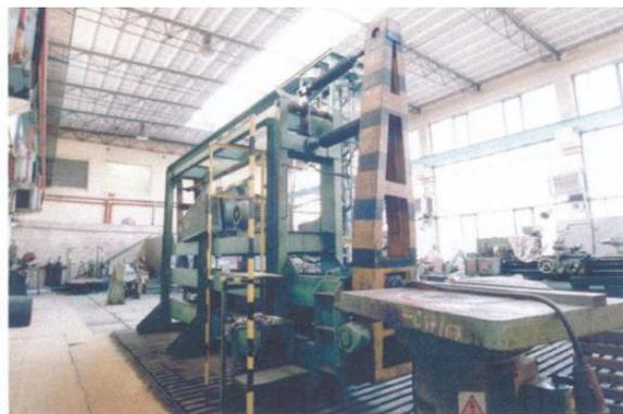
Figure 2. Fatigue machine P5-GIG3 [Zrník 2000, Tomkova 2001]
