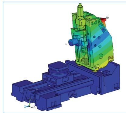
Figure 19. Movable column of the machine tool X-motion axis and its first eigenmode with parallelogram deformation.
