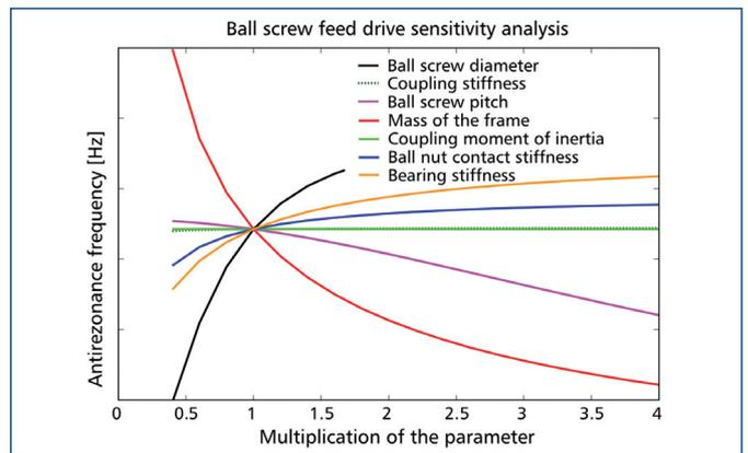
Figure 21. Sensitivity analysis of the first antiresonance frequency to the parameters of the ball screw feed drive components.
