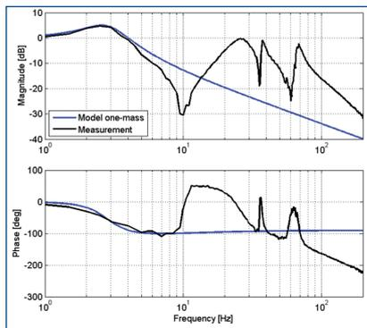
Figure 5. Frequency characteristic of velocity control loop.
