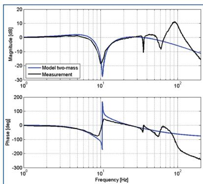
Figure 12. Frequency characteristic of velocity control loop.
