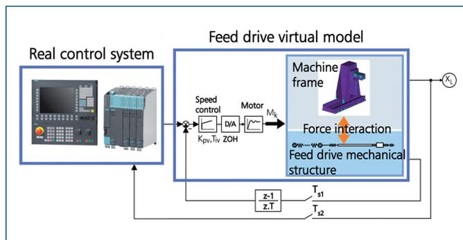
Figure 24. Scheme of the Hardware in the Loop system.
