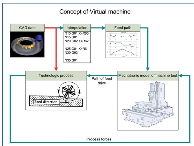
Figure 25. Concept of virtual machine with process model
