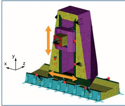
Figure 22. Machine frame FEM model with two movable axes.
