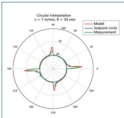
Figure 23. Circular interpolation. Simulation and comparison with measurements.
