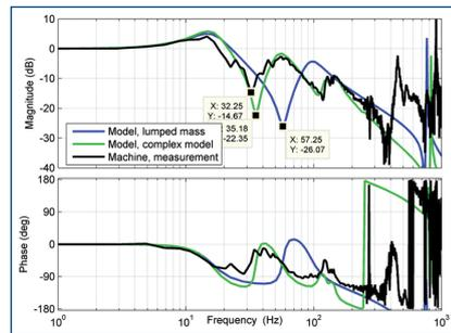
Figure 20. Bode plot of the velocity loop. Comparison of the model with lumped mass representation of movable column, FEM based complex model and real measurements.
