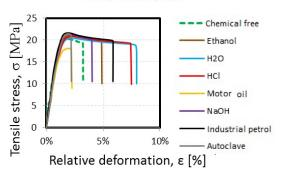
Graph 1. Dependence of the relative deformation on tensile stress for ABS material
