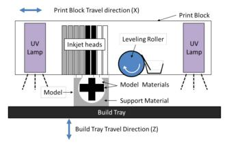
Figure 2. Principle of the PolyJet technology [Gaynor 2014]
