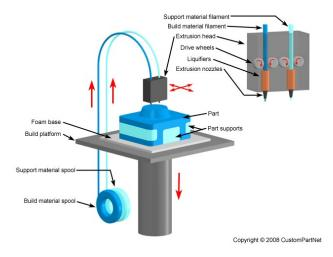
**Figure 1.** Principle of the FDM technology [Custompartnet.com 2015]
