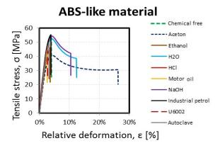
Graph 3. Dependence of the relative deformation on tensile stress for ABS-like material
