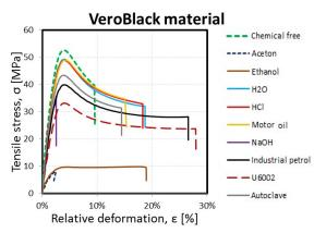
Graph 8. Dependence of the relative deformation on tensile stress for VeroBlack material
