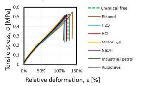
**Graph 7.** Dependence of the relative deformation on tensile stress for TangoBlack+ material
