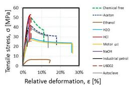
**Graph 9.** Dependence of the relative deformation on tensile stress for VeroWhite material
