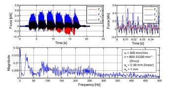
**Figure 10.** Measured cutting forces in time (overview and detail) and frequency domain as result of alternating spindle speed and linear changed immersion [Berthold 2016a].
