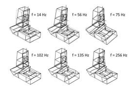
Figure 2. Selected mode shapes at several eigenfrequencies [Putz 2016].
