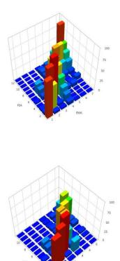
**Figure 17** Comparison mode shapes identified by EMA and OMA using the MAC, left: OMA using EFDD, right: OMA using UPC Merged Data Sets
