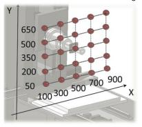
Figure 3. FRF measurement points in the X<sub>NC</sub>-Y<sub>NC</sub>-plane [Putz 2016].
