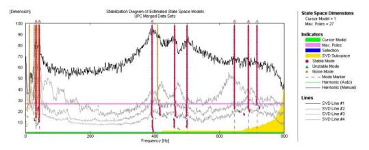
Figure 16Singular values of spectral density matrices estimated by UPC Merged Data Sets [Berthold 2016b]
