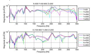
**Figure 4.** Measured FRF in the x-direction for several machine positions [Putz 2016].
