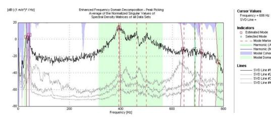
Figure 15. Singular values of spectral density matrices estimated by EFDD [Berthold 2016b]
