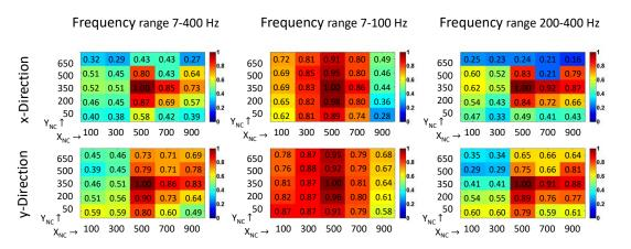
Figure 5. FARC values (also highlighted by colours) in x- and y-direction for different frequency ranges at various machine positions. The reference point for comparison is at  $Z_{NC}$ =500,  $Y_{NC}$ =350,  $Z_{NC}$ =200 [Putz 2016].
