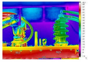
Figure 3. Example of thermogram (biogas plant 1 – transformer object)
