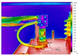
Figure 9. Example of thermogram (biogas plant 3 - transformer object)
