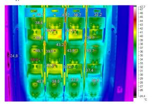
Figure 5.: Example of thermogram (biogas plant 2 - control room)
