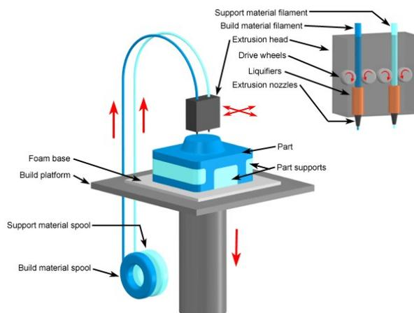
Figure 1. Principle of the FDM technology [Custompartnet.com 2015]
