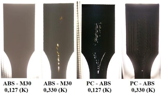
Figure 8. Different specimens' appearance with concentric layer layout
