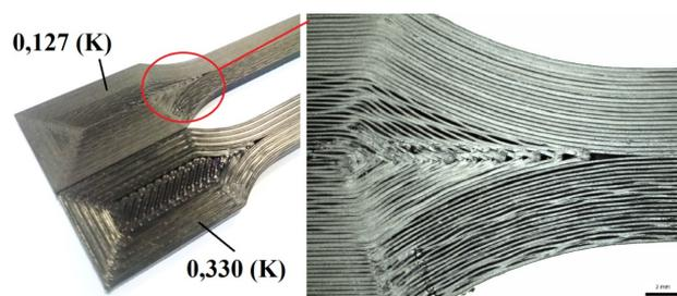
Figure 9. Appearance with concentric layer layout of specimens made of PC / ABS
