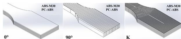
Figure 2. Fibre orientation of printed specimens
