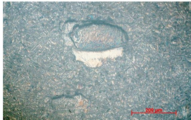
Figure 10. Microscopic image of VeroWhitePlus photopolymer after thermal loading
