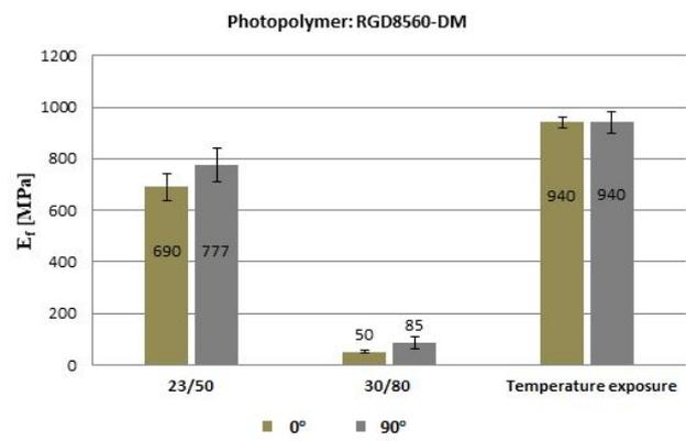
Figure 14. Flexural modulus of RGD8560-DM
