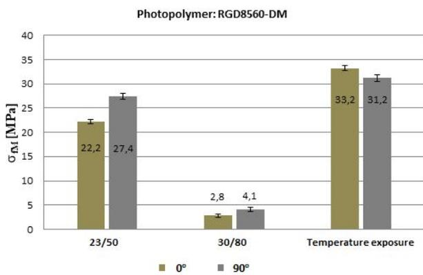
Figure 12. Flexural strength of RGD8560-DM
