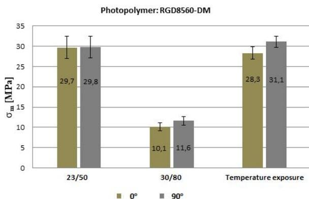
Figure 8. Tensile strength of RGD8560-DM
