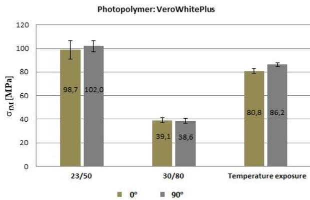
Figure 11. Flexural strength of VeroWhitePlus
