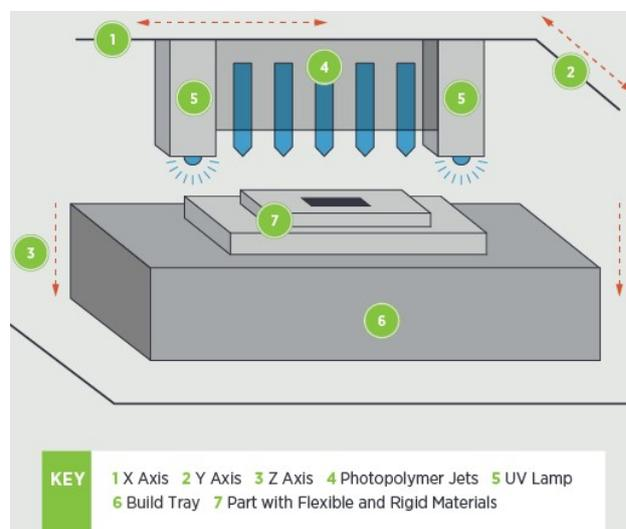
Figure 1. The principle of PolyJet technology [Prolabs 2018]
