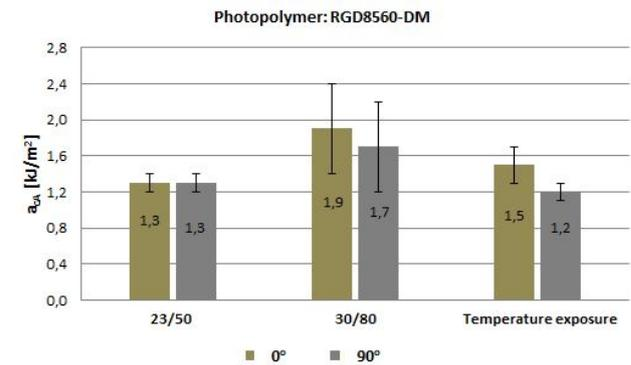
Figure 5. Charpy notched impact strength of RGD8560-DM
