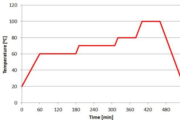
Figure 3. The temperature profile during part conditioning
