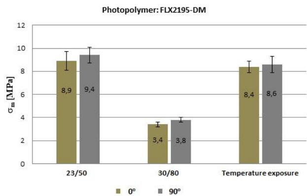
Figure 9. Tensile strength of FLX2195
