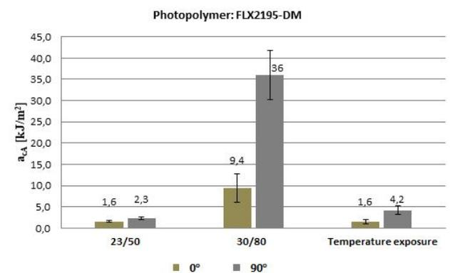
Figure 6. Charpy notched impact strength of FLX2195-DM
