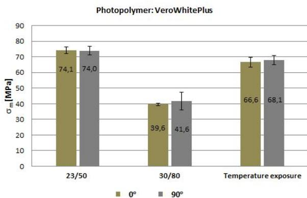
Figure 7. Tensile strength of VeroWhitePlus
