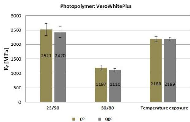
Figure 13. Flexural modulus of VeroWhitePlus
