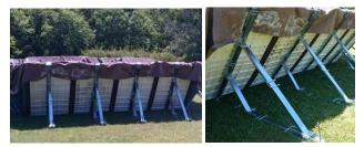
Figure. 10 Modular flood barrier structure – test basin at TOP 2016
