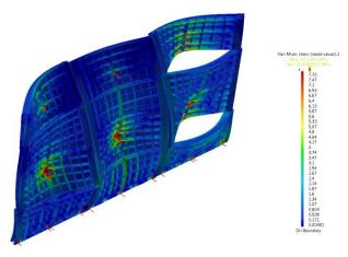
Figure 4. Finite element method FEM analysis of the arrangement of plastic block loading [MPa]
