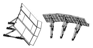
Figure 1. Modular flood barrier structure
