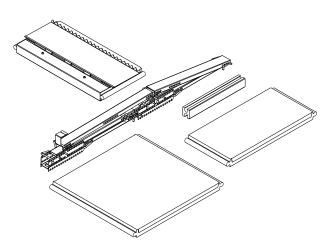
Figure 11. Basic parts of the modular structure of walls in disassembled state before assembly
