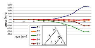
Figure 8. Illustration of the results of the tensometric measurement of stress, in dependence on the watter level [Soos 2014a]
