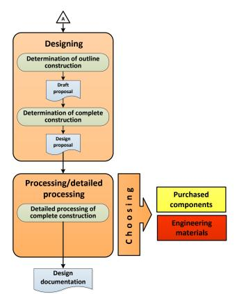
Figure 2. Design process of machinery [Blecha 1999] (to be continued)
