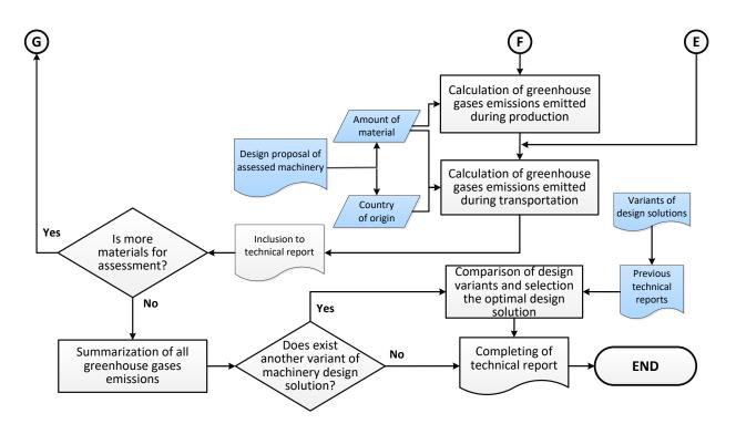
Figure 4. Methodology for assessment of GHG emissions released throughout production of engineering materials (to be continued)
