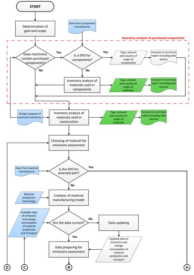
Figure 4. Methodology for assessment of GHG emissions released throughout production of engineering materials
