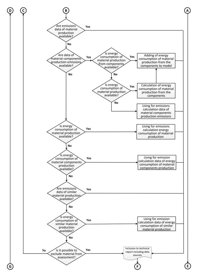
Figure 4. Methodology for assessment of GHG emissions released throughout production of engineering materials (to be continued)
