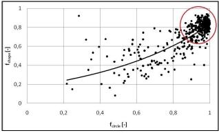
Figure 7. Dependence f<sub>circle</sub> vs. f<sub>shape</sub>. In red circle are ideal shape pores
