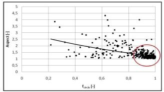
Figure 9. Dependence  $f_{\text{circle}}$  vs. Aspect. In red circle are pores that are close to the ratio of 1
