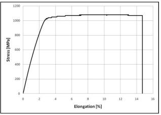
Figure 4. Diagram from the static tensile test
