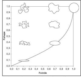
Figure 2. The pores shapes in depending on f<sub>shape</sub> and f<sub>circle</sub>.
