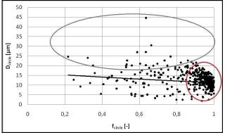
Figure 8. Dependence  $f_{\text{circle}}$  vs.  $D_{\text{circle}}$  . In red circle is the average pore size. In gray circle are pores with a higher diameter
