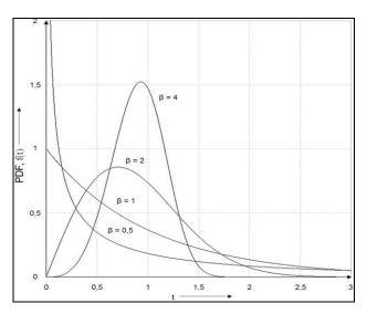
Figure 3: Weibullprobability density function, cf [Jiang 2006]
