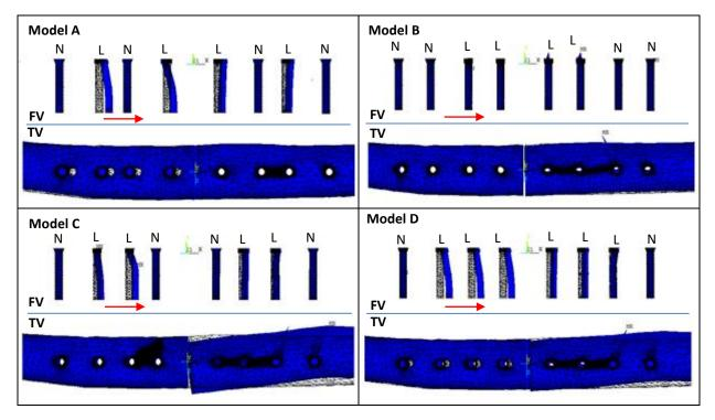
Figure 12. Simulation of the approximation displacements that occur when hybrid plating subjected to axial loading. The meshed volume is the actual shape and the blue color is the displaced volume. The red arrow indicates bending forces direction. FV: front view, TV: top view, correspond to the modelling coordinate system on Fig.7.
