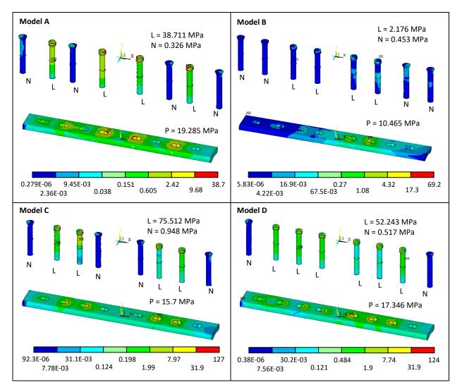
Figure 9. Contour plot of stress on hybrid models plating; L denotes for locking screw, N is nonlocking screw, and P is locking plate (von Mises stress in MPa)
