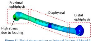
Figure 11. Plot of stress contour on internal fixation of Model A
