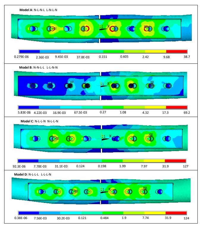
Figure 8. Stress distribution on fracture femur with hybrid plating fixation under axial loading (von Mises Stress in MPa)
