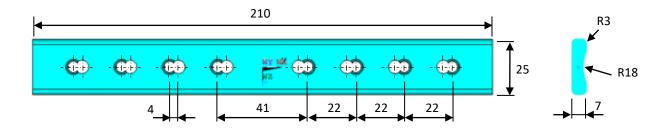
Figure 2. Dimensions of LCP plate with 8 screw holes configuration (in mm)
