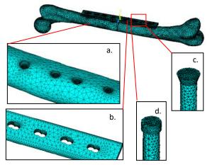
**Fig. 5.** Meshed volume on femur fracture with internal fixation model; (a) femur bone, (b) locking plate, (c) locking screw and (d) nonlocking screw.
