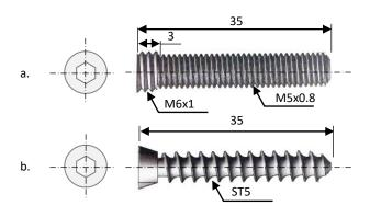
Figure 3. Dimensions of bone screw; (a) locking screw (b) nonlocking screw [Synthes 2002] (in mm)
