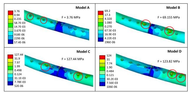
Figure 10. The contour plot of stress distribution on the femur bone (von Mises stress in MPa). Red circles indicate the maximum stress sites.
