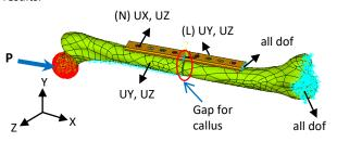
**Figure 7.** Boundary conditions applied on femur fracture with internal fixation. UX, UY, and UZ means constrained displacements in X, Y, and Z direction, respectively, and all dof means all degree of freedom is constrained.
