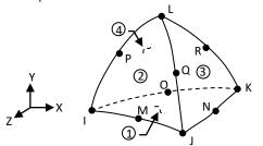
**Fig. 4.** Geometry of SOLID187 elements. I, J, K, L, M, N, O, P, Q and R are denoting the node numbers at their corresponding position. 1, 2, 3 and 4 represent the surface coordinate systems which are related to the surface load [ANSYS 2017]
