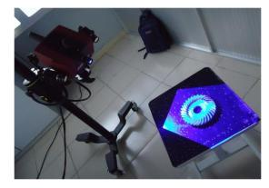
Figure 6. Scanning the machined gear.
