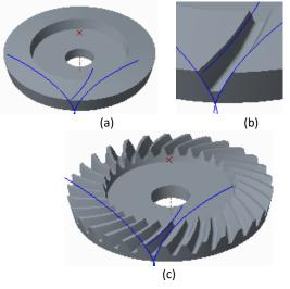
Figure 1. Some basic steps for modelling the designed gear.
