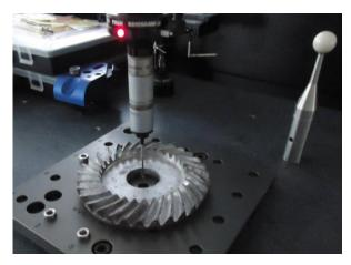
Figure 8. Measuring single pitch error on the Smart CMM.
