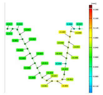
Figure 7. Detailed deviations of some tooth profiles.
