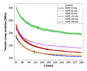
Figure 8. Tensile-creep modulus of irradiated HDPE
