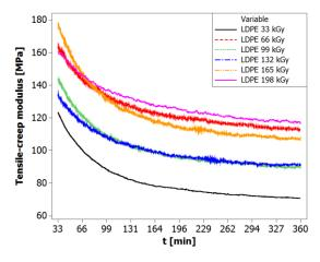
Figure 7. Tensile-creep modulus of irradiated LDPE
