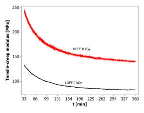
Figure 6. Tensile-creep modulus of HDPE and LDPE
