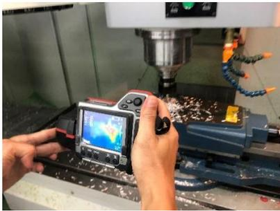
**Figure 15.** Temperature measurement on the surface of the tool outside the cutting zone using a thermal scanning camera
