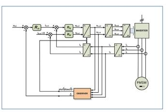
Figure 1. The sensorless drive structure used in a study
