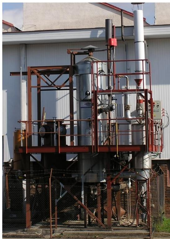
Figure 1. Atmospheric fluidized bed gasifier Biofluid design
