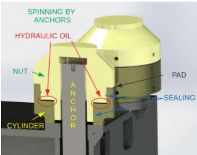
Figure 3. Spinning by anchors
