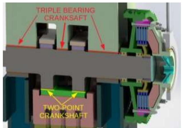
Figure 7. Triple bearing crankshaft, Two-point crankshaft
